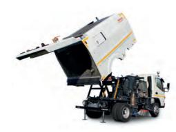
The special high tipping technology allows raising the debris hopper to 1.50 m and emptying it in a provided container.
